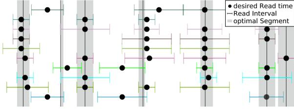
**Figure 3: Plot of optimal time frames for sensor reads and selected read times with ten concurrent queries on the public transport dataset.**
