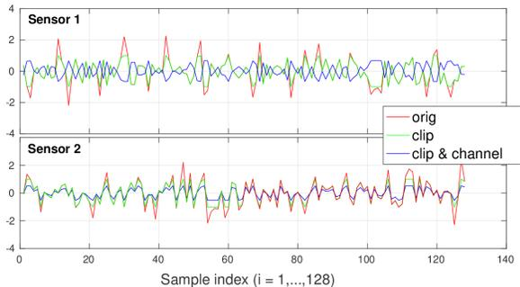
Fig. 2. Transmitted signals of the first two sensors  $j = 1, 2$ : The original signal (red), clipped channel input (green) and clipped channel output (blue). Note that the first sensor is affected by a sign change, i.e.,  $\text{sign}(h_j) = -1$ .
