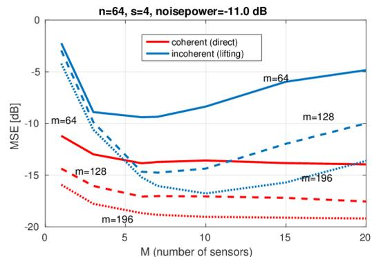
Fig. 3. Mean squared error (MSE) for signal reconstruction with coherent (red) and non-coherent transmission (blue) via ( $P_R^{\text{Dir}}$ ) and ( $P_R^{\text{Lift}}$ ), respectively.
