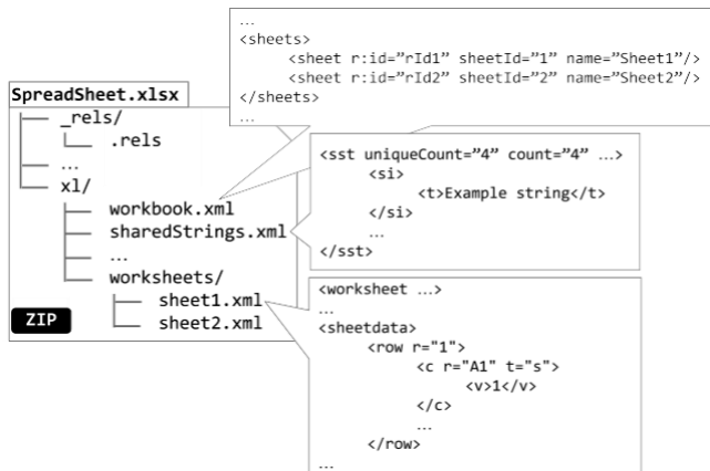
Fig. 3. Spreadsheet structure (simplified).
