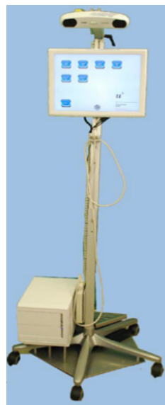
Figure 1: The soft-tissue navigation system CASOne from CASCination GmbH, Switzerland. (Image taken from Matthias Peterhans et al. [PDN + ]. For more information about the system please refer to their web page [CAS].)
