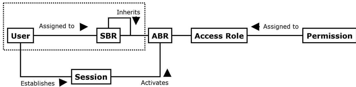
Fig. 2: UML Class Diagram: Distributed RBAC Model
