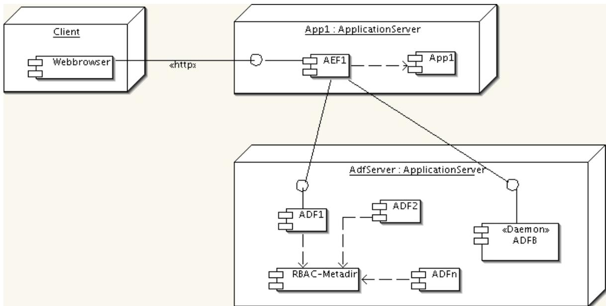
**Fig. 5:** UML Deployment Diagram: Isolated ADF-Components
