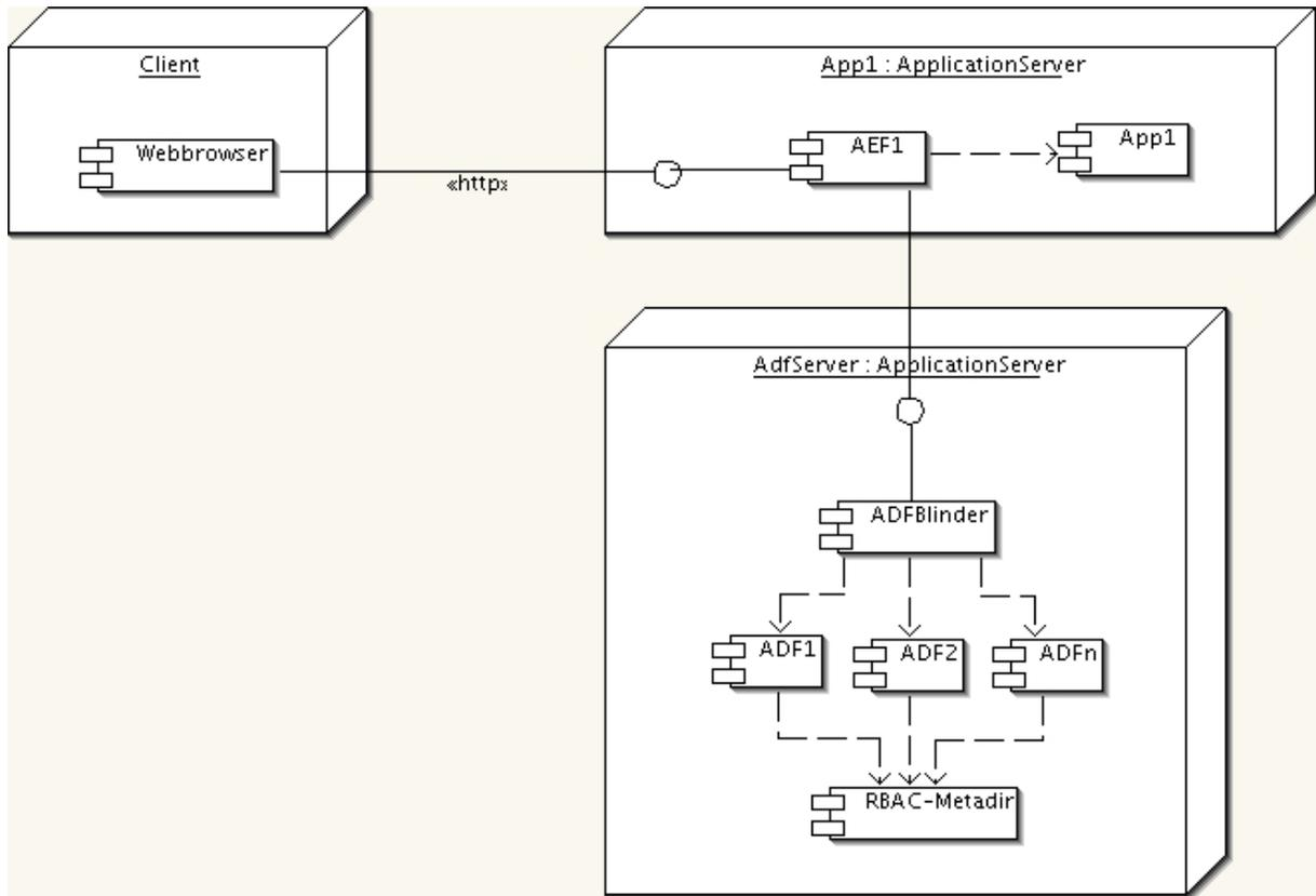
**Fig. 3:** UML Deployment Diagram: ADFBlinder Architecture
